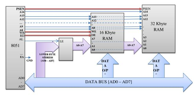
The lower order address and data bus are multiplexed. De-multiplexing is done by the latch. Initially the address will appear in the bus and this latched at the output of latch using ALE signal. The output of the latch is directly connected to the lower byte address lines of the memory. Later data will be available in this bus. Still the latch output is address it self. The higher byte of address bus is directly connected to the memory. The number of lines connected depends on the memory size.
